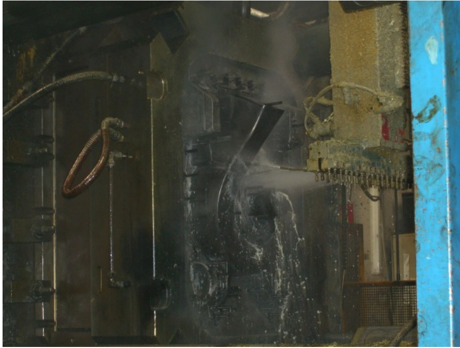
Choosing the best release agent is a vital contributor to trouble-free production.. Photo courtesy Fondermetal SPA, Sotto Il Monte, Italy.
