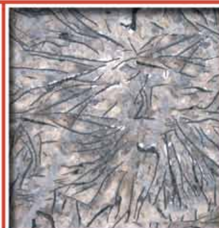
Gray Cast Iron Attack Nital 4%
