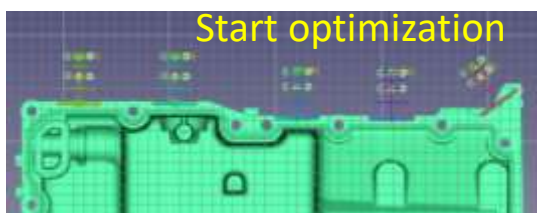
QuickCAST analysis for engine block (Gravity casting)
