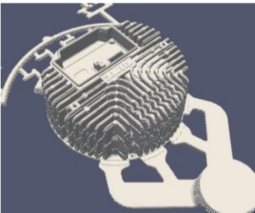
Tradition FDM mesh (in 1,298,853 cells)
